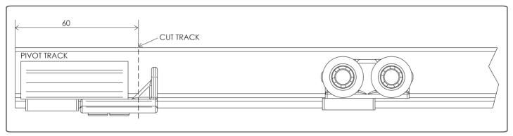
NOTE: YOU CAN EITHER INSTALL TRACK WITH HARDWARE ALREADY INSIDE TRACK OR CUT A 60 MM SECTION OFF THE END TO FEED HARDWARE IN AFTER FITTING THE TRACK INTO THE FRAME.
