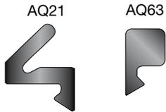
**31a** Stick the 2pc self adhesive seals QL3116BLK onto the top and bottom pivot hinge plate on Door 1 pivot door and Door 4 Access Door (4pc seals). Ensure the self adhesive seals are applied in line with the AQ21 in the door.
