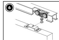
Hook the door onto the runners using the door brackets fixed to the top of the door. Insert the under door profile over the door guide and slide into the pocket. There is one adjustable stop already installed 70 mm from
