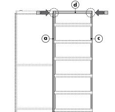
Assemble the pocket header (d) to the central verticals (a) and rear verticals (c) using 4.2 x 9.5 mm screws (m).
