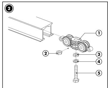
Assemble both runners (1) using a runner nuts (2), lock nuts (3), washers (4) and bolts (5) as shown and insert into the overhead track at the doorpost end.
