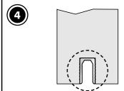
Cut the Under Door Profile to 10 mm longer than the door width. Route a channel 10,3 x 17 mm into the bottom of the door from the rear of the door to the 5 mm from the front edge of the door. Using a small amount of silicon insert the under door profile into the channel. It should protude 15 mm at the rear of the door.
