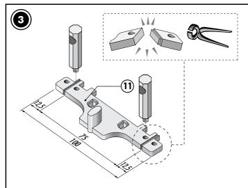
Only if you have a 100 mm finished wall thickness then you need to break off the ends of the guide base (11). Insert the posts into the holes on the guide and attach to the frame at the pocket entrance at finished floor level using the self-drilling screws (12).
