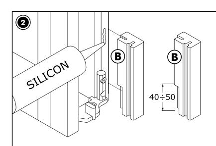
Trim the lower position of the vertical pocket jamb (B) to accommodate the guide and attach to both sides of the pocket entrance using 4/5 blobs of silicon.
