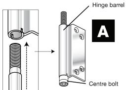
17 Fix top and bottom pivot hinges to door 1 using screws supplied in premachined positions.
