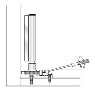
Insert pivot base into cill channel. Drill pilot hole in channel and fix with self-tapping screw.
