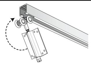
7b Slide the intermediate carrier wheels into the track.
