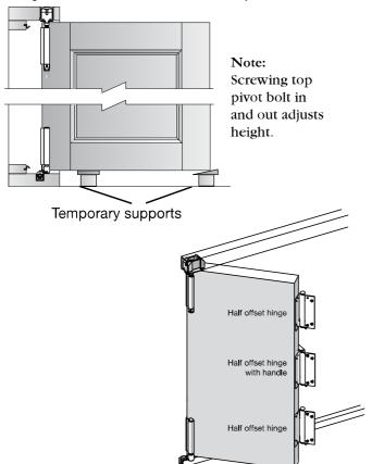
Adjust alignment of pivot door as shown. Leave a 7mm gap between the door edge and the frame jamb.
