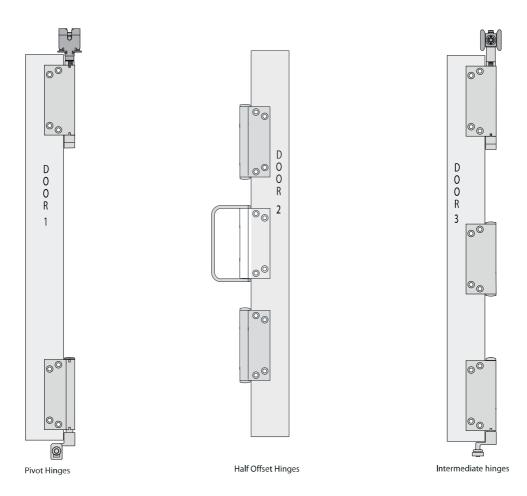
Note: Pivots are reversible. The pivots are delivered set up for this option 'B' - Use without change.
