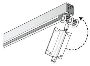
**7a** Slide the intermediate carrier wheels into the track.
