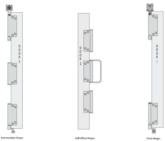
Note: Pivots are reversible. For this option 'A' it is necessary to take the top and bottom pivots apart to reverse them - see 16
