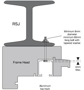
The aluminium top track, which is temporarily held in place with transit screws, has been pre-drilled for fixing points into the Lintel.
