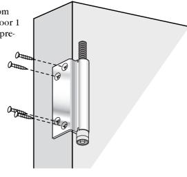
Assemble top pivot block. Slide and click cover plate onto the pivot block. Screw through cover plate into rear of access slot ensuring the pivot block is sitting tight up against the frame jamb.
