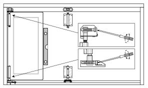
Fit half offset hinges to the inside edge of door 1. in the machined position using screws provided.
