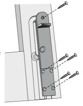
15 Fit the keyed drop bolt cup to the cill in the pre-cut position.
